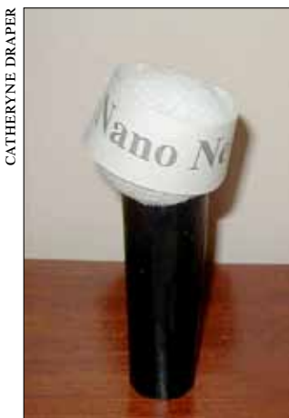
The mic is made of a cutoff paper roll wrapped in black plastic and topped off with a styrofoam ball.
